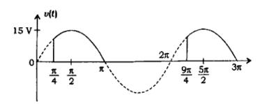
Determine (i) the average value and (iii) the r.m.s. value of the voltage. 10
